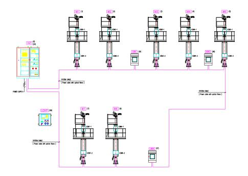
This diagram is a schematic representation of a system composed by 7 monitor, 3 fixed and 1 portable command and control panel.
