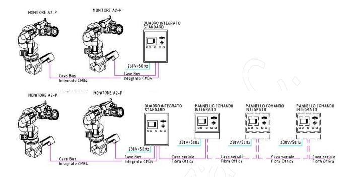
In conclusion, command of A2 monitors is possible, for all their functions of elevation, rotation, nozzle and valve,
