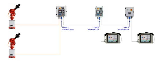
The same portable unit can be mounted on more sockets, or more portable units can be connected at the same time to more sockets.
