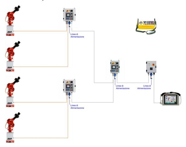
The limit of 4 monitors in the system depends only on the use of the standard command panels.
