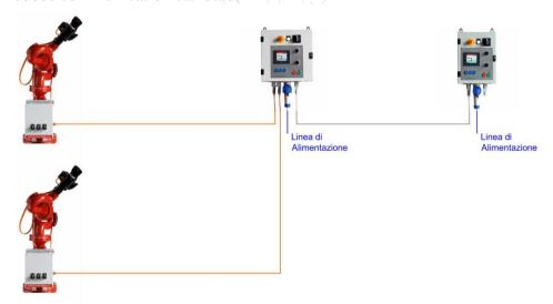
The max. length of the connecting cable is 250 m. (In case of necessity, longer distances, even kms, can be covered using customized (not standard) panels.
