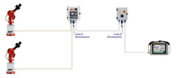
Other standard remote command panels and/or other panels with socket for portable units can be mounted in sequence to the first standard remote command panel (or alternatively to the panel with socket without commands).
