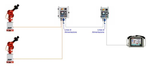
The alternative to the remote panel with socket for portable command is a panel without commands, but equipped only with the special socket for connection of the portable command unit.
