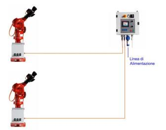
An additional remote command panel can be connected to the power and command panel. The connection between the two panels is performed by means of a single cable according to modbus communication standard.
