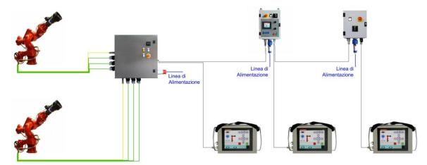
Other standard remote command panels and/or other socket panels for portable units can be mounted in sequence to the first standard remote command panel (or alternatively to the socket panel without commands).
