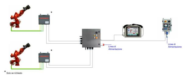
An additional remote command panel can be connected to the power and command panel. The connection between the two panels is performed by means of a single cable according to communication standard modbus or ethernet.
