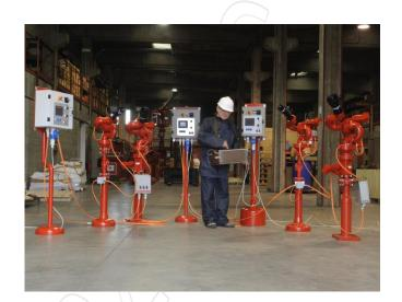
The monitors A3, A4, A6 and A8 types are available also in Ex-proof execution for mounting in hazardous areas where explosions may be caused either by gas or powder.
