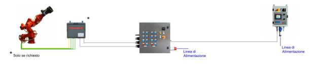
In any case the power panel is equipped with a special socket for direct connection of a portable command unit by means of a mobile cable whose max. length is 30 m.
