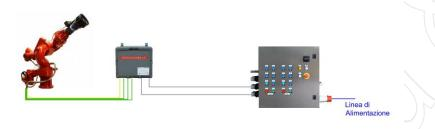
Monitor commands can be placed in a control panel separate from the power panel. The power panel can be equipped also with local commands, or not, as required. In the same way there can be or not the terminal cabinet between the monitor and the power panel according to the requirements.
