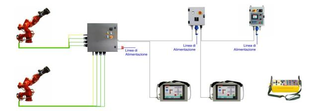
The portable panels with radio connection have all the functions available for the other command panels.
