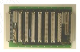
to an MOT24 board by means of connectors in order to extend the control unit's bus.
