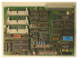
command by means of the MOT14 and MOT15 boards. This card is also interfaced to the display, in order to show the statuses of all the system components, and to the alphameric keyboard in order to enter commands.
